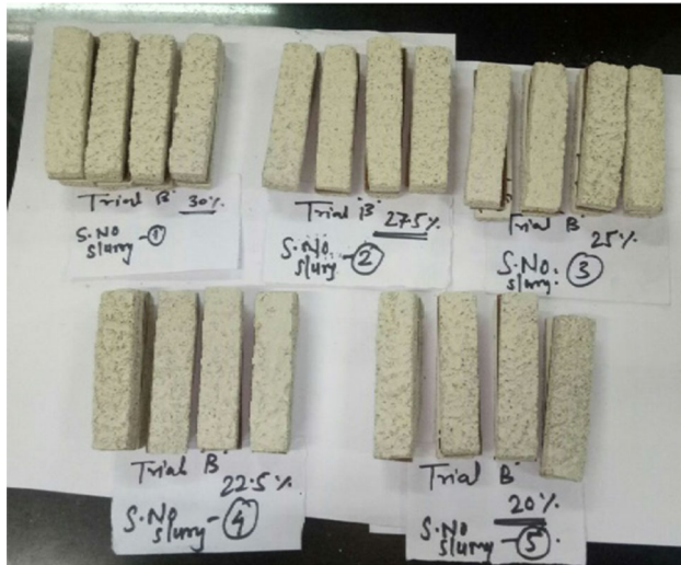
Fig. 2 Test piece for modulus of rupture
