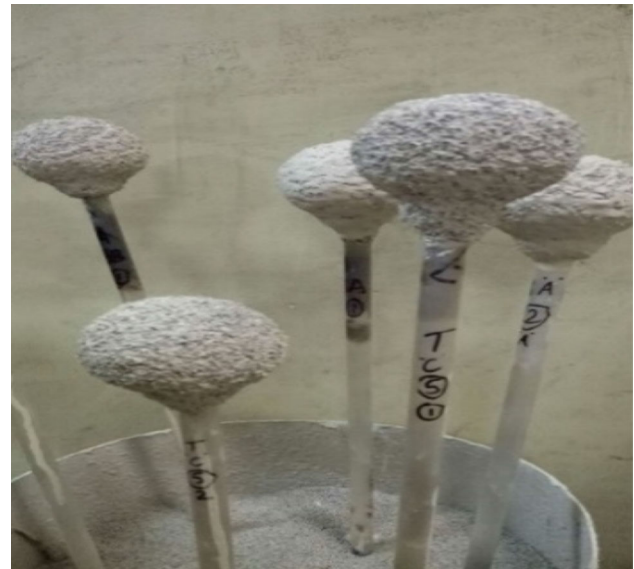
Fig. 3 Test piece for permeability
