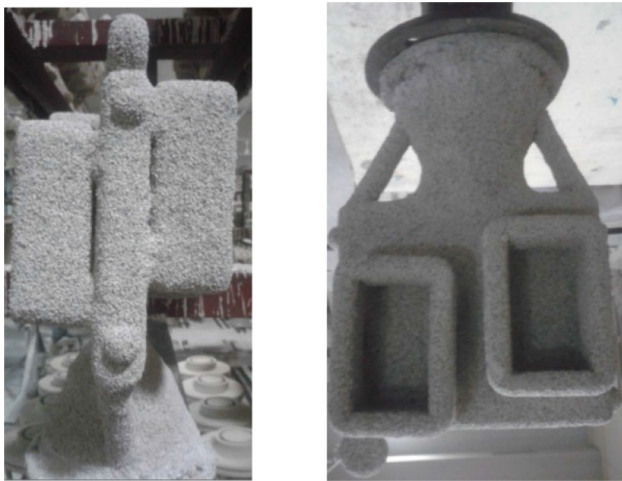
Fig. 7 Shell mould for component
